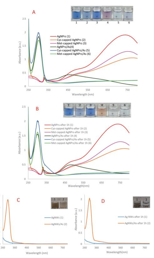
Fig. 1 The UV-Vis spectra of sensing probes in the presence and absence of arsenic (A) AgNPrs, Cys-capped AgNPrs, Met-capped AgNPrs; (B) AgNPrs, Cys-capped AgNPrs, Met-capped AgNPrs after 1 h; (C) AgNWs and (D) AgNWs after 1 h.
