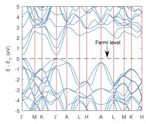
Fig. 2 The band structure of  $\text{Cu}_3\text{P}$  from the PBE functional with Hubbard potentials. The gap opened up with value of 0.41 eV. However, the band curvatures are almost identical to without Hubbard
