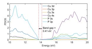
Fig. 3 The PDOS plot of  $Cu_3P$  with Hubbard potentials (22, 18). The gap value of 0.41 eV was obtained as it was in the band structure diagram using the same Hubbard values.
