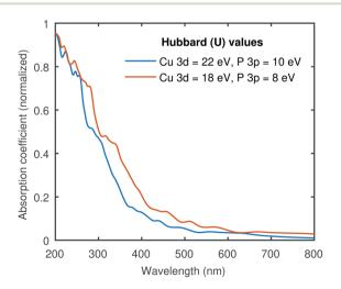
Fig. 5 The absorption coefficient of  $Cu_3P$  at two different sets of Hubbard values. The results are qualitatively similar to the expected shift across the x-axis due to the difference in the band gap.
