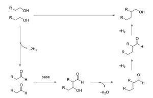
Fig. 8 Plausible reaction pathway for Guerbet reaction with DMF-stabilized Ru NPs.
