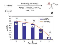
Fig. 4 DMF-stabilized Ru NP reuse in Guerbet reaction of 1-octanol.
