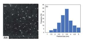
Fig. 1 (a) ADF-STEM image of DMF-stabilized Ru NPs and (b) particle size distribution.
