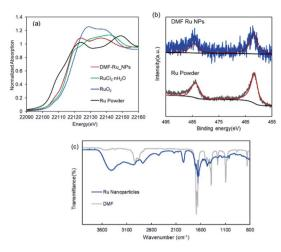
Fig. 2 (a) Ru K-edge XANES spectra of DMF-stabilized Ru NPs (red),  $RuO_2$ , and Ru powder; (b) Ru 3p XPS spectra of DMF-stabilized Ru NPs (blue) and Ru powder (gray); and (c) FT-IR spectra of DMF-stabilized Ru NPs (blue) and DMF (gray).
