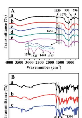
Fig. 7 FT-IR spectra of (A) BMMs-based samples. (a) Pure mesoporous materials, (b) Zn-modified samples, (c)  $Z_1$ -immobilized samples, (d)  $Z_2$ -immobilized samples, and (e)  $Z_3$ -immobilized samples, in which the molar ratios of Z/Zn for all samples were around 1 : 1. (B-a)  $Z_1$ , (B-b)  $Z_2$ , and (B-c)  $Z_3$ .
