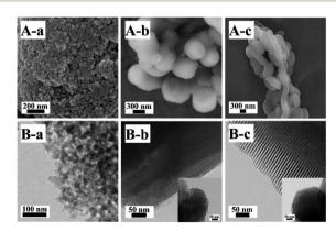
Fig. 5 SEM (A) and TEM (B) images of (a) Z<sub>2</sub>ZnBMMs-100, (b)  $Z_2ZnMCM-41-100$ , and (c)  $Z_2ZnSBA-15-100$ . Inset shows a TEM image of the sample viewed along the hexagonal axis.
