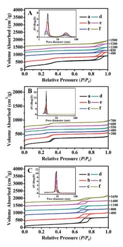
Fig. 4  $N_2$  adsorption—desorption isotherms and corresponding pore size distribution (inset) of (A) BMMs-, (B) MCM-41-, and (C) SBA-15-based samples. (a) Pure mesoporous materials, (b) Zn-modified samples, (c) Z<sub>1</sub>-immobilized samples, (d) Z<sub>2</sub>-immobilized samples, and (e) Z<sub>3</sub>-immobilized samples, and (f)  $3^{rd}$  recycled Z<sub>2</sub>-immobilized samples, in which the molar ratios of Z/Zn for all samples were around 1:1.
