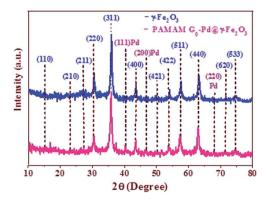
Fig. 2 XRD patterns of  $\gamma\text{-Fe}_2\text{O}_3,$  and PAMAM  $\text{G}_0\text{-Pd}@\gamma\text{-Fe}_2\text{O}_3$  complex.
