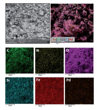
Fig. 5 EDS elemental mappings of the PAMAM  $G_0\text{-Pd}@\gamma\text{-Fe}_2O_3$  complex.
