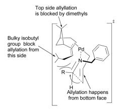
Fig. 8 Proposed transition state of (–)- $\beta$ -pinene-based  $\pi$ -allylpalladium mediated allylation of imine.
