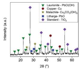
Fig. 1 X-ray diffractogram of starting material.
