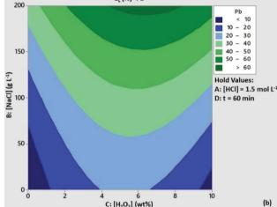
Fig. 4 Contour plots of Pb leaching efficiency as a function of (a) [HCl]/[NaCl] and (b) [ $H_2O_2$ ]/[NaCl]. Conditions: L/S = 10 mL g $^{-1}$ , T=80 °C, t=60 min and (a) [ $H_2O_2$ l] = 10 wt%, (b) [HCl] = 1.5 mol L $^{-1}$ .
