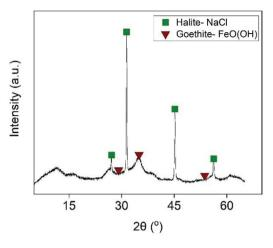
Fig. 10 X-ray diffractogram of the iron-rich precipitate.
