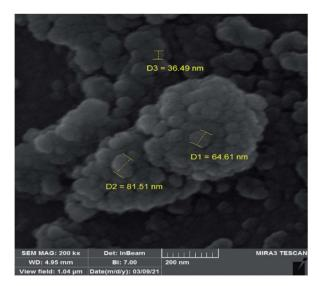
Fig. 11 SEM image of the recovered catalyst.
