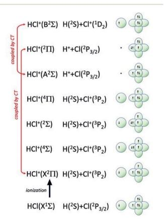
Fig. 7 Symmetry of the ground state of HCl molecule and sequence of molecular states accessible to HCl<sup>+</sup> molecular ion. The asymptotic correlation with the states of atomic partners involved in the molecular bond is also represented. The energies of most relevant atomic and molecular states are given in absolute scale in Fig. 9.
