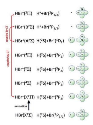
Fig. 8 Symmetry of the ground state of HBr molecule and sequence of molecular states accessible to HBr<sup>+</sup> molecular ion. The asymptotic correlation with the states of atomic partners involved in the molecular bond is also represented. The energies of most relevant atomic and molecular states are given in absolute scale in Fig. 9.
