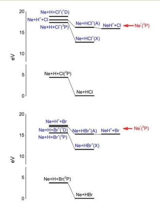
Fig. 9 Energy levels of neutrals and ionic species involved in CHEMI of HCl and HBr with metastable  $Ne*(^3P)$  atoms. See also Fig. 7 and 8 for the symmetry of the states.
