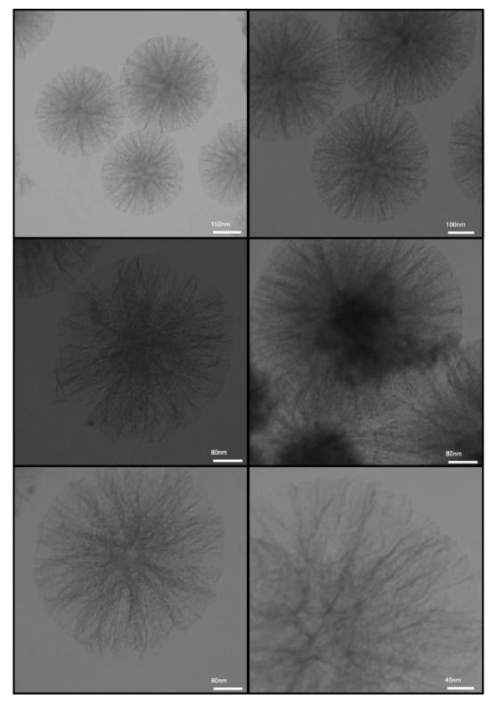
Fig. 5 TEM images of the dendritic Fe<sub>3</sub>O<sub>4</sub>@SiO<sub>2</sub>@KCC-1@MPTMS@Cu<sup>II</sup> nanocomposite.
