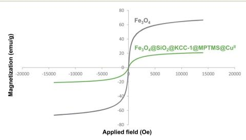
Fig. 8 VSM diagram of the  $Fe_3O_4$  NPs and  $Fe_3O_4$ @SiO<sub>2</sub>@KCC-1@MPTMS@Cu<sup>II</sup> nanocomposite.
