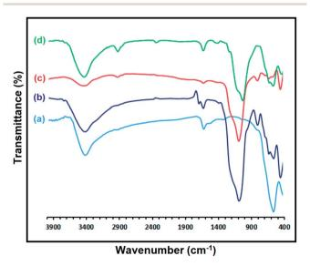
Fig. 2 FT-IR spectra of the (a)  $Fe_3O_4$ , (b)  $Fe_3O_4$ @SiO<sub>2</sub>@KCC-1, (c)  $Fe_3O_4$ @SiO<sub>2</sub>@KCC-1@MPTMS, and (d)  $Fe_3O_4$ @SiO<sub>2</sub>@KCC-1@MPTMS@Cu<sup>II</sup> nanosystems.
