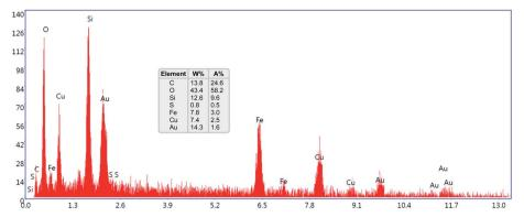
$\label{eq:Fig.6} \textbf{Fig. 6} \quad \text{SEM-based EDX spectrum of the } \text{Fe}_3\text{O}_4\text{@SiO}_2\text{@KCC-1@MPTMS@Cu}^{\text{II}} \text{ nanocomposite.}$
