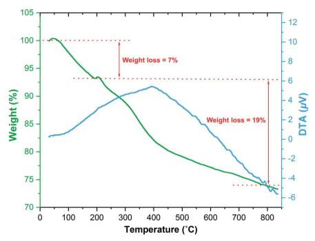
$\label{eq:Fig.7} \textbf{Fig. 7} \quad \textbf{TGA/DTA diagram of the } \text{Fe}_3\text{O}_4\text{@SiO}_2\text{@KCC-1}\text{@MPTMS}\text{@Cu}^{II} \text{ nanocomposite.}$
