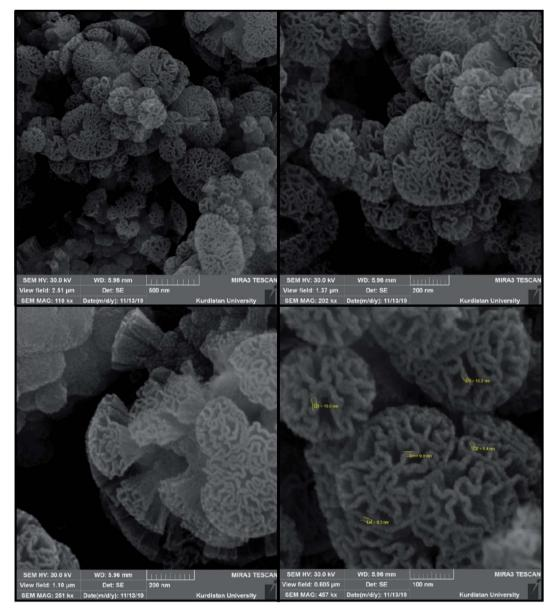
Fig. 4 SEM images of the cockscomb flower-like Fe<sub>3</sub>O<sub>4</sub>@SiO<sub>2</sub>@KCC-1@MPTMS@Cu<sup>II</sup> nanocomposite.
