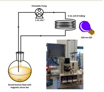
Fig. 6 Schematic representation of the continuous flow set up used to reduce the time required for the Minisci-type reaction. Inset picture shows the Easy-Photochem flow system from Vapourtec equipped with the UV-150 photoreactor.
