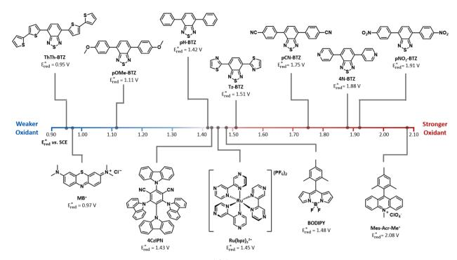
Fig. 3 Comparison between the excited state reduction potentials ( $E_{red}^*$ ) of selected BTZ photocatalysts (above axis) and common photocatalysts discussed in literature (below axis). 27,28,52-54
