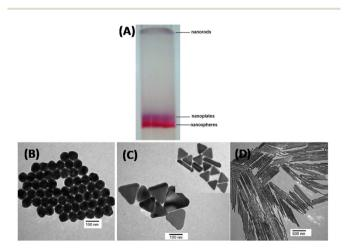
**Fig. 4** (A) Digital image of preparative agarose gel electrophoretic column shows the separated nanospheres (red band), nanoplates (blue band) and long nanorods (light brown band), TEM images of (B) separated pure nanospheres, (C) separated nanoplates (inset shows some short rods coexist with plates), and (D) purified long gold nanorods. This figure has been reproduced from ref. 50 with permission from Elsevier, copyright 2005.
