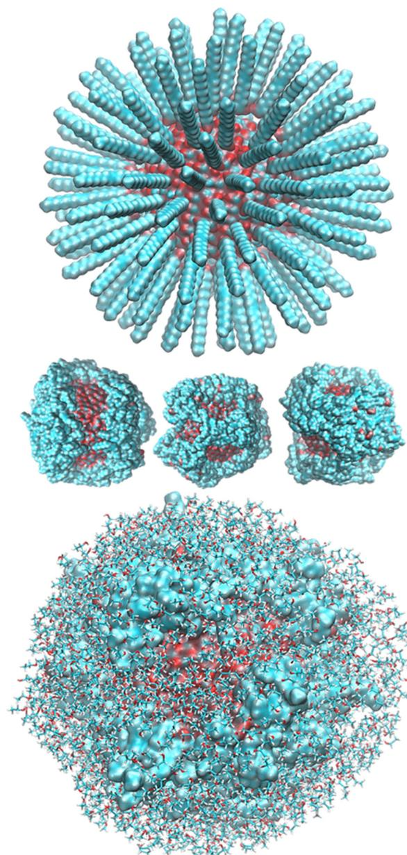
**Fig. 3** Initial and final arrangements of ZnONP functionalized with OLA. In the top and middle images, ETH molecules have been undisplayed for clarity, and in contrast, the bottom image shows them through the stick model. The ZnONP surface has been rendered through the solvent-accessible surface and OLA chains with the vdW representation. Color codes: C cyan, O red, H white, Zn bluish.
