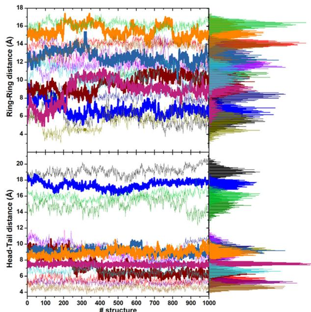
**Fig. 7** Evolution of the ring–ring and head–tail distances of the adsorbed CFZ molecules during the last 200 ps production dynamics in ETH solution. Thicker lines highlight the trends of these descriptors for those molecules directly connected to the ZnO surface. On the right, the distributions are also shown.
