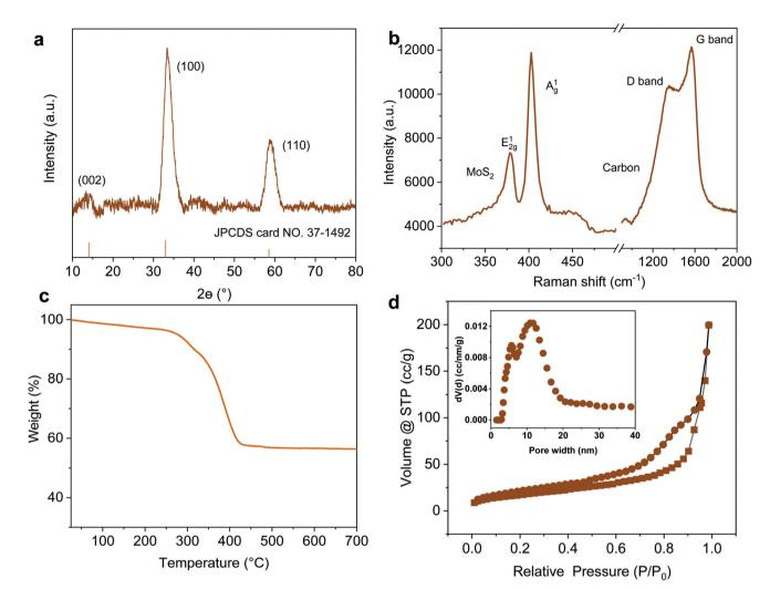
Fig. 3 (a) XRD pattern, (b) Raman spectrum, (c) TGA in air and (d)  $N_2$  adsorption/desorption isotherm curves of MoS<sub>2</sub>-1.5 PNPs; the inset is the curve of pore size distribution.
