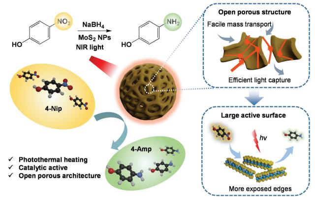
Scheme 2 Schematic of 4-Nip reduction with porous MoS<sub>2</sub> under NIR light illumination.
