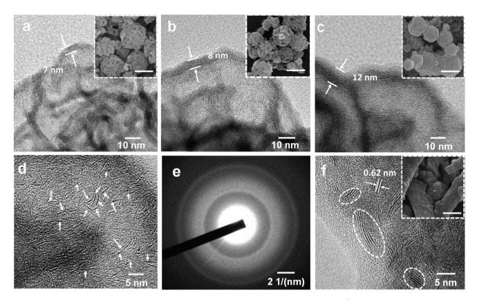
Fig. 2 TEM images of MoS<sub>2</sub> PNPs prepared at precursor concentrations of (a) 1, (b) 1.5, and (c) 3 mg mL<sup>-1</sup>. The insets are the corresponding SEM images with a scale bar of 500 nm. (d) HRTEM image and (e) SAED pattern of MoS<sub>2</sub>-1.5 PNPs. (f) HRTEM image of bulk MoS<sub>2</sub> prepared without any polymer template; the inset is the corresponding SEM image with a scale bar of 500 nm.
