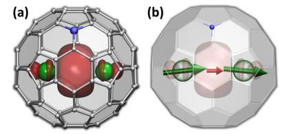
Fig. 1 (a) Molecular structure of Tb<sub>2</sub>@C<sub>79</sub>N with valence spin density isosurface corresponding to the singly-occupied Tb-Tb bonding orbital; Tb is green, N is blue, carbons are grey. (b) Alignment of magnetic moments in  $Tb_2@C_{79}N$ ; green arrows – localized Tb-4f moments, red arrow – unpaired electron spin residing on the Tb-Tb bonding molecular orbital.
