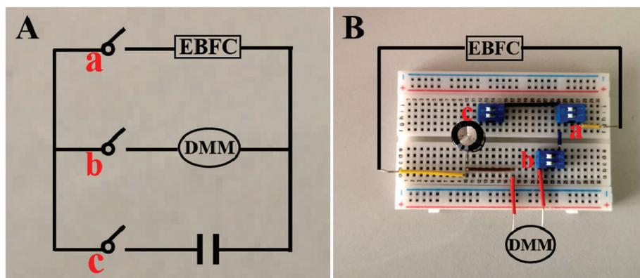
Fig. 1 Photos of circuit diagram (A) and breadboards used for measuring the instantaneous current of the device (B).
