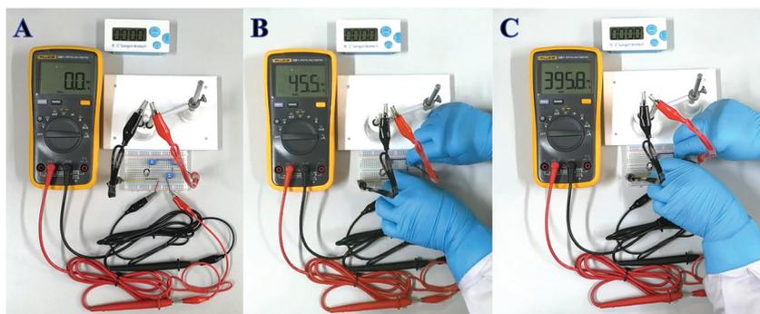
Fig. 8 The optical photographs of uncharged capacitor (A), after incubation with 1 nM miRNA (B), and after charging (C).
