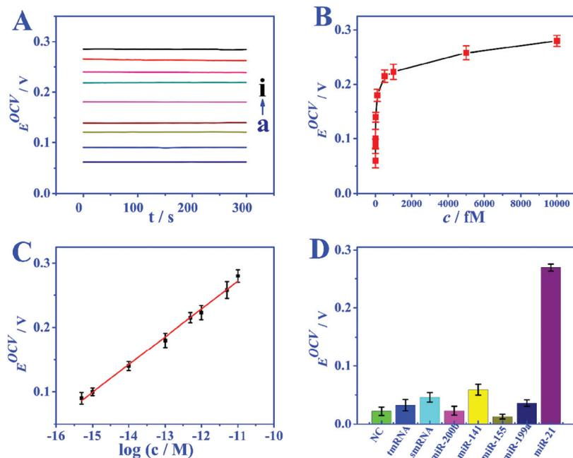
**Fig. 5** (A)  $E^{OCV}$  of the biosensor of miRNA with various levels (a–i: 0, 0.5, 1, 10, 100, 500, 1000, 5000, 10 000 fM). (B) The variation of  $E^{OCV}$  as a function of miRNA concentration. (C) The linear relationship between  $E^{OCV}$  and the logarithm of miRNA-21 concentration from 0.5 to 10 000 fM. (D) Selectivity of the biosensor.
