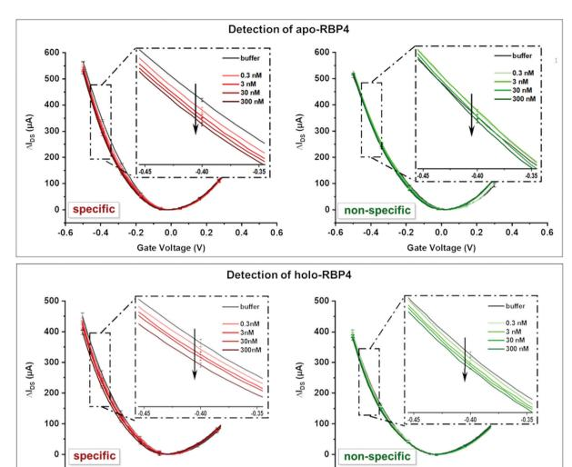
Fig. 3 Top: Detection of apo-RBP4. Bottom: Detection of holo-RBP4.  $I_DV_G$  curves are an average of a minimum of 3 individual curves with error bars showing the standard deviation. Both devices showed significantly more pronounced shifts in their  $I_DV_G$  characteristics upon specific analyte binding.
