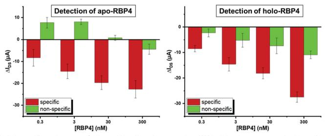
Fig. 4 Average difference in current at -0.4 V upon addition of increasing concentrations of RBP4.  $\Delta$ -Values shown are averages of a minimum of three independent experiments on different devices. Error bars show the standard deviation.
