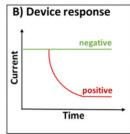
Scheme 3 (A) Typical configuration of an EG-FET. (B) Response of the device when there is no target analyte (green) and when the target analyte is present (red)
