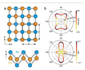
Fig. 1 (a) Top and side views of the FeAs monolayer, where the unit cell is represented by the black rectangle. The orange and blue balls are Fe and As atoms, respectively. (b) Angular dependence of the Young's modulus  $Y(\theta)$  and Poisson ratio  $\nu(\theta)$  of the FeAs monolayer, where the angle  $\theta$  is defined relative to the x-direction.
