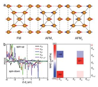
Fig. 2 (a) The ferromagnetic configuration and two types of antiferromagnetic configurations of the FeAs monolayer. Only the Fe atoms are shown here for clarity. (b) The projected density of states (PDOS) of Fe-d orbitals and orbital resolved MAE of the FeAs monolayer. 'O' and 'U' represent occupied and unoccupied states, respectively.
