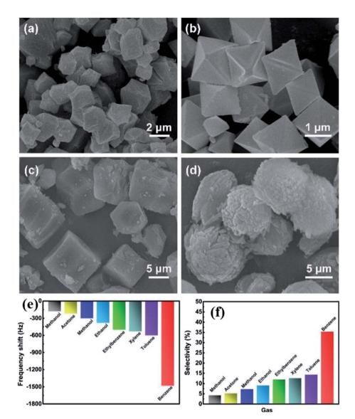
Fig. 20 FESEM images of the as prepared MOFs: (a) MOF-14, (b) HKAUST-1, (c) MOF-177, and (d) MOF-74, (e) response profile of the MOF-14based QCM sensor towards different VOCs for 100 ppm benzene at 25C°C, and (f) selectivity study of the MOF-14-sensor in different interfering gases towards 100 ppm benzene at RT. Reproduced from ref. 163 with permission from Elsevier, copyright 2021.
