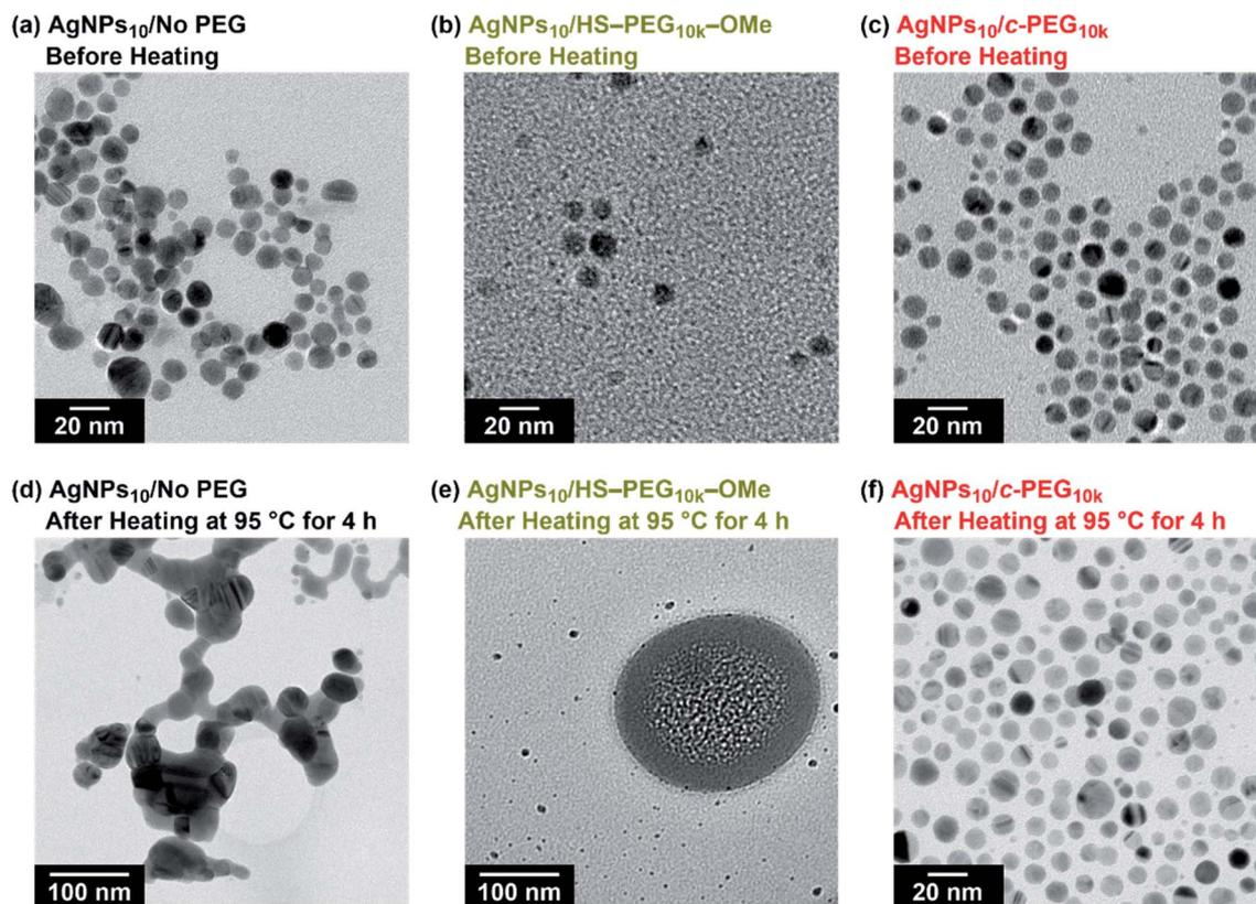
Fig. 6 TEM photographs of (a) AgNPs<sub>10</sub>/No PEG (scale bar: 20 nm), (b) AgNPs<sub>10</sub>/HS-PEG<sub>10k</sub>-OMe (scale bar: 20 nm), and (c) AgNPs<sub>10</sub>/c-PEG<sub>10k</sub> (scale bar: 20 nm) before heating. Those of (d) AgNPs<sub>10</sub>/No PEG (scale bar: 100 nm), (e) AgNPs<sub>10</sub>/HS-PEG<sub>10k</sub>-OMe (scale bar: 100 nm), and (f) AgNPs<sub>10</sub>/c-PEG<sub>10k</sub> (scale bar: 20 nm) after heating at 95 °C for 4 h.
