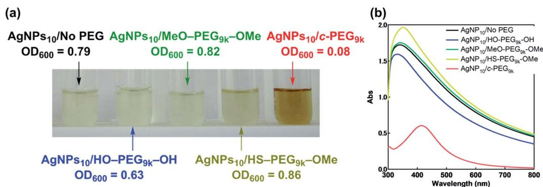
Fig. 7 (a) Photograph and (b) UV-Vis spectra of the antimicrobial efficacy test against *E. coli* after 24 h of incubation with AgNPs<sub>10</sub>/No PEG, AgNPs<sub>10</sub>/HO-PEG<sub>9k</sub>-OH, AgNPs<sub>10</sub>/MeO-PEG<sub>9k</sub>-OMe, AgNPs<sub>10</sub>/HS-PEG<sub>9k</sub>-OMe, and AgNPs<sub>10</sub>/c-PEG<sub>9k</sub>. UV-Vis spectra of the incubated specimens subtracted by that of the medium are shown.
