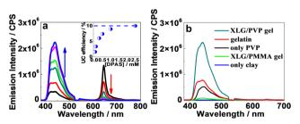
Fig. 3 (a) UC emission intensities as a function of DPAS concentrations in the XLG/PVP gel at room temperature ([PtOEP] = 10  $\mu$ M); inset: UC quantum yields as a function of DPAS concentrations. Note: the blue arrow stands for the increase of UC intensity, and the red arrow stands for decreased the intensity of the phosphorescence of PtOEP. (b) UC emission intensity of 2.5 mM **DPAS** and 10  $\mu$ M **PtOEP** in different hydrogels. ( $\lambda_{ex}$  = 532 nm, P.I. = 8 mW).
