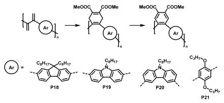
Fig. 9 Post-polymerisation functionalisation of a diene-containing polymer via Diels-Alder reaction. Four different aromatic units were incorporated in the main chain of the conjugated polymer. After Diels-Alder reaction, the polymers were rearomatized in an additional step. 82
