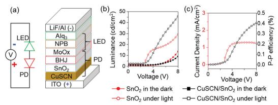
Fig. 3 Upconversion imagers with different interlayers in the photodiode stack. The incident light was at an intensity of 5 mW cm<sup>-2</sup> from a 1050 nm light source. (a) Schematics of the upconversion imager with the CuSCN/SnO2 bilayer. (b) Luminance of the visible light emitted from the imager versus the applied bias. (c) Current density and photon-to-photon upconversion efficiency versus the applied bias.
