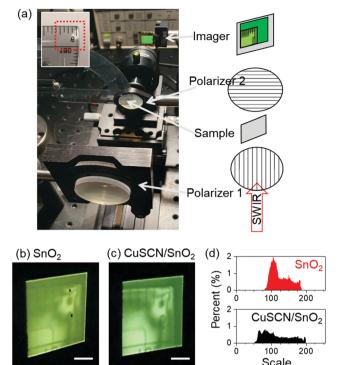
Fig. 4 Results of upconversion images. (a) Imaging setup. The red box on the plastic protractor indicates the area being imaged. Upconversion images produced by (b) the imager with conventional interlayer and (d) the imager with the heterojunction interlayer. The scale bar represents 5 mm. The imagers were operated at 5 V, and the sample was under 290  $\mu$ W cm<sup>-2</sup> illumination from a 940 nm LED. (d) Histograms of images in parts (b) and (c).
