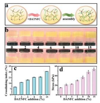
(a) The illustration of the self-assembly process, (b) optical photos, (c) crosslinking indexes and (d) tensile stress of GDH.
