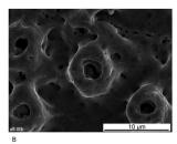
Fig. 4 (A) Scanning electron microscopy (SEM) image of a hydrophilic SLA surface (SLActive, Institute Straumann AG, Basel, Switzerland). There are no distinct differences in specific SEM features between hydrophilic and standard SLA surfaces. (B) SEM images of an anodically oxidized Ti surface (TiUnite, Nobel Biocare, Zürich, Switzerland) displaying protruded open pore micro-structures.
