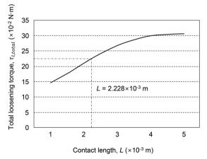
Fig. 11 The effect of contact length, L, on the total loosening torque,  $\tau_{\text{Ltotal}}$ . This graph shows total loosening torque values, based on the data in Table 1
