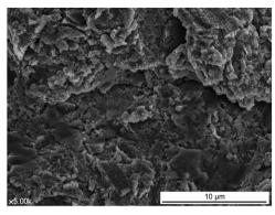
Fig. 6 Image of a fluoride-treated surface (Osseospeed, Astra Tech, Dentsply, Waltham, MA, USA). After blasting with Ti dioxide particles, the surface is treated with fluoride. Consequently, the surface is similar to those blasted with Ti dioxide particles alone.
