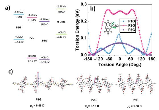
Fig. 1 Results from DFT calculations. (a) energy levels of CPs and N-DMBI (b) torsion energy profiles of the NDI-R<sub>2</sub> bond. (c) Energy minimized 3D structure and dipole moments of the backbone of tetramer models for CPs, arrows are vectors depicting the magnitude and direction of the dipole moment
