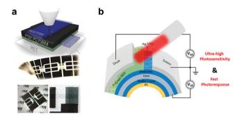
(a) Schematic structure and photographs of fully-printed ITO-free OPDs on PET foil showing their semi-transparency and mechanical flexibility.<sup>216</sup> (b) Device structure of flexible PT-OPDs with ultrashort channel length. 217 (a) Reproduced with permission.<sup>216</sup> Copyright 2015, WILEY-VCH GmbH. (b) Reproduced with permission.<sup>217</sup> Copyright 2018, American Chemical Society.
