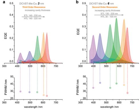
Fig. 9 EQE curves and correlated FWHM of cavity enhanced OPDs with (a) 3 nm thick photo-absorbing layer and third order resonance (m = 3) and (b) 6 nm thick photo-absorbing layer and second order resonance (m = 2). The tunable enhanced wavelengths are realized by varying the thickness of ETL and HTL. Reproduced with permission.<sup>81</sup> Copyright 2019, American Chemical Society.
