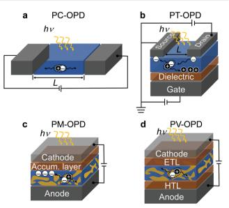
Fig. 1 Schematic of organic electronic device architectures for photodetection. (a) Organic photoconductor (PC-OPD); (b) organic phototransistor (PT-OPD); (c) photomultiplication type OPD (PM-OPD), in this example an accumulation (accum.) layer is inserted to block electrons; and (d) photovoltaic type OPD (PV-OPD) with an electron (ETL) and hole transport layer (HTL).
