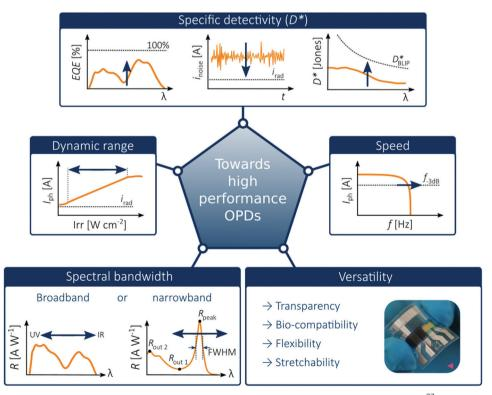
Fig. 2 Illustration of challenges for emerging OPDs. The picture of the flexible OPD is reproduced with permission,<sup>27</sup> copyright 2017, Springer Nature.
