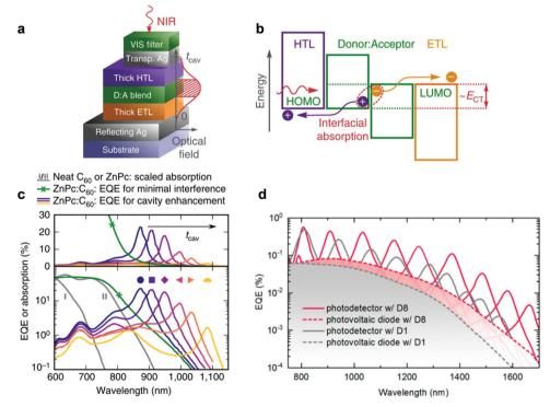
Fig. 10 (a) Simplified device architecture of a microcavity enhanced narrowband NIR OPD. (b) Schematic energy level diagram of the main materials involved in the OPDs. (c) NIR OPDs based on ZnPc: $C_{60}$  CT state absorption. (d) NIR OPDs based on the CT absorption of D8: $C_{60}$ . Subfigures (a–c) are reproduced with permission.<sup>27</sup> Copyright 2017, Springer Nature. Subfigure (d) is reproduced with permission.<sup>197</sup> Copyright 2019, American Chemical Society.
