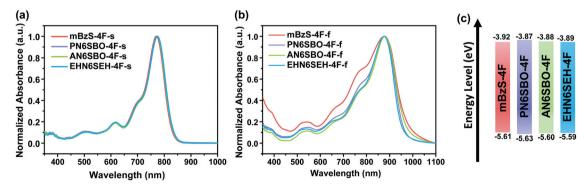
Fig. 2 Normalized UV-vis absorption spectra of mBzS-4F, PN6SBO-4F, AN6SBO-4F and EHN6SEH-4F measured as (a) dilute solutions in CHCl<sub>3</sub> and (b) thin-films. (c) Frontier orbital energy levels of mBzS-4F, PN6SBO-4F, AN6SBO-4F and EHN6SEH-4F.
