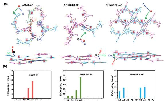
Fig. 4 (a) Top view and side view of the labeled nearest-neighbor molecules in the single-crystal structures of mBzS-4F, AN6SBO-4F and EHN6SEH-4F. (b) Electronic coupling between the nearest neighbors.
