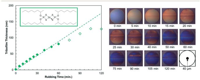
Fig. 2 Representative example (oct-2-yl ZDDP at 80 °C and 1000 N) of the tribofilm thickness growth over time, measured from the SLIM images shown on the right. Dashed linear fits are used to calculate the growth rates (filled symbols only). Black circle (diameter = 40 µm) represents the area over which the mean tribofilm thickness was measured in the central region of the contact.
