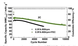
Fig. 5 Long-term galvanostatic cycling of LTO  $\parallel$  NMC $_{532}$  full-cells without (in black) and with FEC as electrolyte additives (in green). Following two formation cycles at 0.1C, the cells were subjected to constant current cycling at a dis-/charge rate of 2C. The cut-off potentials were set to 1.4 V and 2.8 V.
