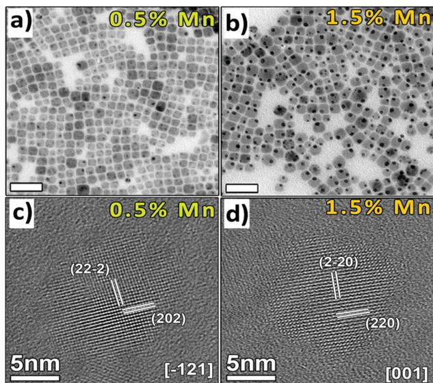
Fig. 13 TEM images of (a) 0.5% and (b) 1.5% and HRTEM images of (c) 0.5% and (d) 1.5% Mn-doped  $\text{Cs}_2\text{AgInCl}_6$  NCs respectively. Reproduced with permission.<sup>84</sup> Copyright 2018, American Chemical Society.
