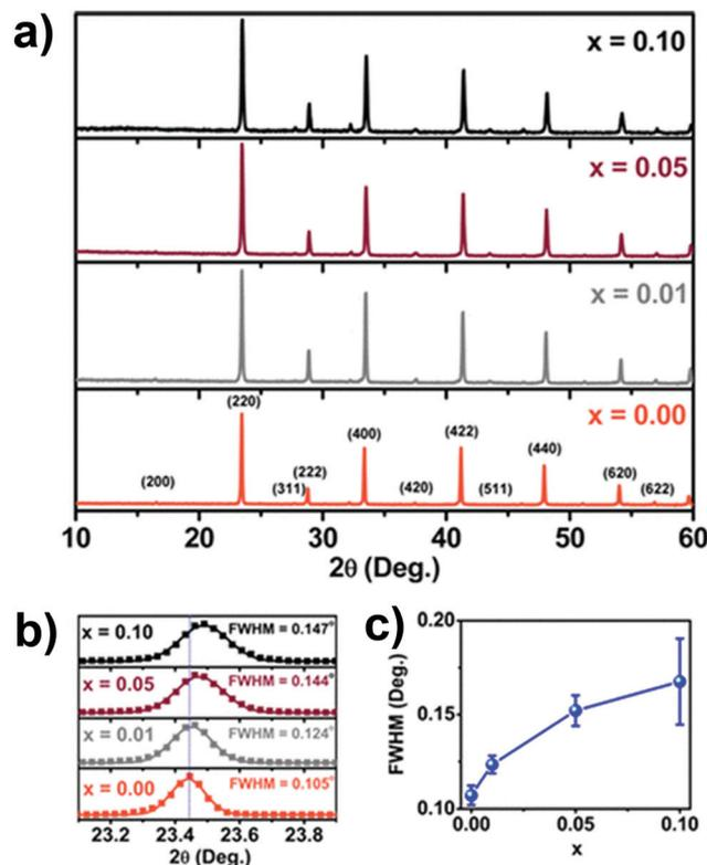
Fig. 5 (a) XRD patterns of undoped and Cu doped  $\text{Cs}_2\text{AgSbCl}_6$  MCs, (b) expansion of the (220) plane in the XRD patterns and (c) broadening of the FWHM. Reproduced with permission.<sup>80a</sup> Copyright 2018, American Chemical Society.
