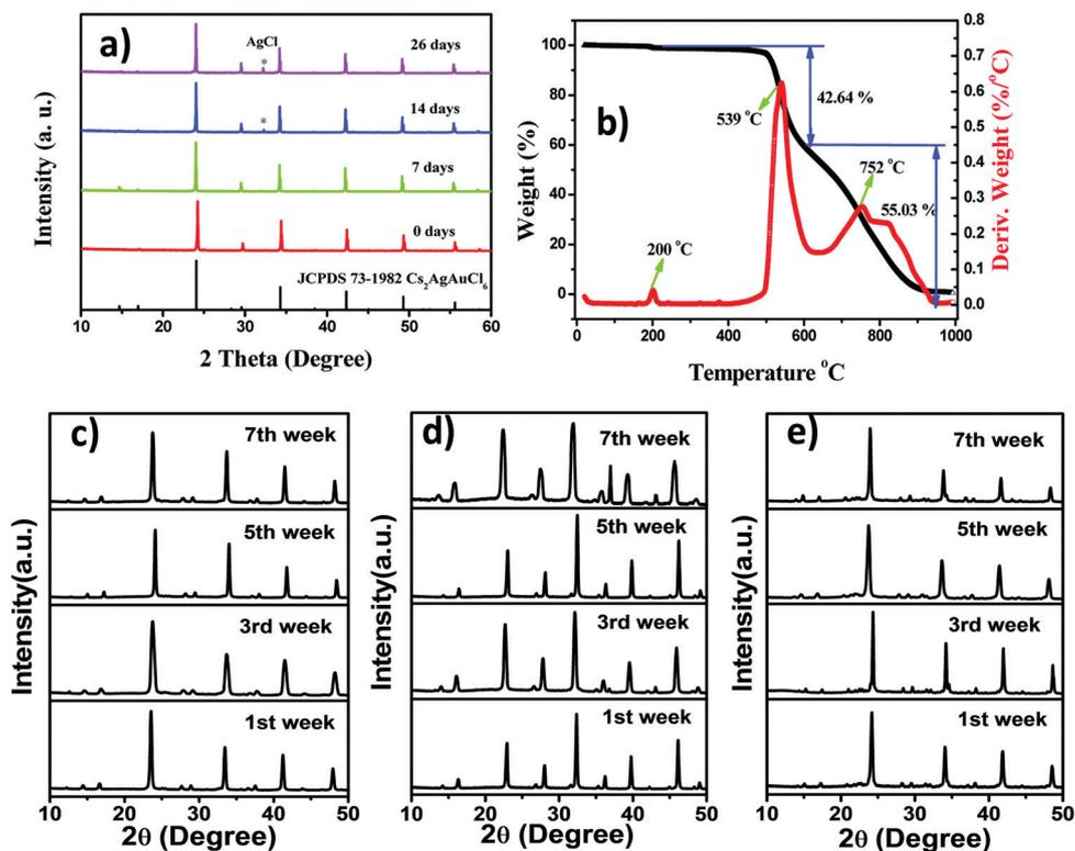
Fig. 15  $\text{Cs}_2\text{AgInCl}_6$  MCs: (a) P-XRD patterns at 7, 14 and 26 day intervals, and (b) TGA and DSC curves. Reproduced with permission.<sup>79</sup> Copyright 2017, Royal Society of Chemistry. P-XRD patterns of (c)  $\text{Cs}_2\text{AgBiCl}_6$  MCs and (d)  $\text{Cs}_2\text{AgBiBr}_6$  MCs in organic medium, and (e)  $\text{Cs}_2\text{AgBiBr}_6$  MCs in a mixture of aqueous and organic media. Reproduced with permission.<sup>76</sup> Copyright 2021, Elsevier.
