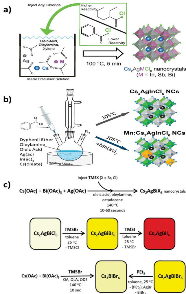
Fig. 6 Synthesis of (a) metal halide double perovskite nanocrystals. Reproduced with permission.<sup>83</sup> Copyright 2019, American Chemical Society. Synthesis of (b) undoped and Mn doped  $\text{Cs}_2\text{AgInCl}_6$  nanocrystals. Reproduced with permission.<sup>84</sup> Copyright 2018, American Chemical Society. (c)  $\text{Cs}_2\text{AgBiX}_6$  nanocrystals via an anion exchange method. Reproduced with permission.<sup>86</sup> Copyright 2018, American Chemical Society.
