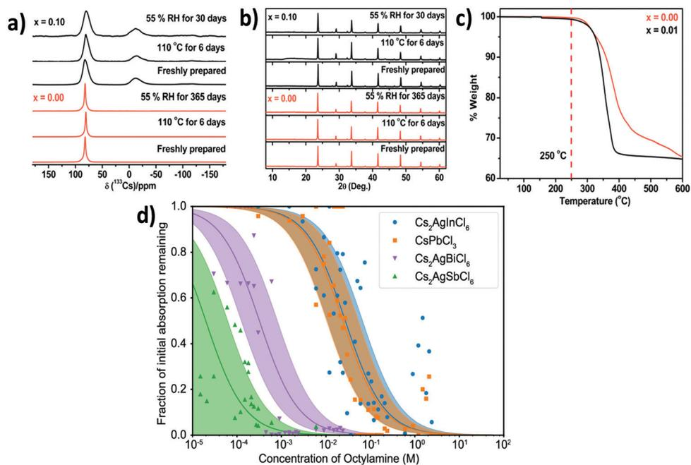
Fig. 16 (a) NMR, (b) P-XRD and (c) TGA spectra of undoped and Cu doped  $\text{Cs}_2\text{AgSbCl}_6$  MCs. Reproduced with permission.<sup>80a</sup> Copyright 2018, American Chemical Society. (d) Stability analysis of  $\text{Cs}_2\text{AgSbCl}_6$ ,  $\text{Cs}_2\text{AgInCl}_6$ ,  $\text{Cs}_2\text{AgBiCl}_6$  and  $\text{CsPbCl}_3$  NCs by amine titration. Reproduced with permission.<sup>83</sup> Copyright 2019, American Chemical Society.
