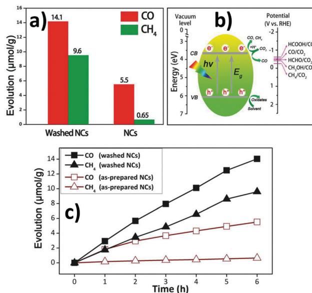
Fig. 20 (a) Comparison of the performance of CO<sub>2</sub> reduction between the as-prepared and washed Cs<sub>2</sub>AgBiBr<sub>6</sub> nanocrystals, (b) photo-reduction of CO<sub>2</sub> on the surfaces of the nanocrystals, and (c) time courses of CO and CH<sub>4</sub> evolution. Reproduced with permission.<sup>103</sup> Copyright 2018, Wiley-VCH.
