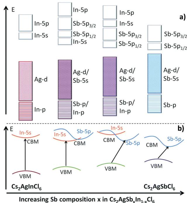
Fig. 10 (a) Schematic diagram of the bonding and antibonding orbitals of  $\text{Cs}_2\text{AgSb}_x\text{In}_{1-x}\text{Cl}_6$  and (b) transition from direct to indirect bandgaps on changing the character of the VBM and CBM. Reproduced with permission.<sup>90</sup> Copyright 2017, Royal Society of Chemistry.
