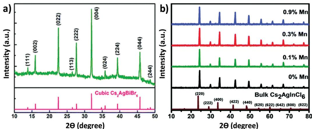
Fig. 4 XRD pattern of (a) the Cs<sub>2</sub>AgBiBr<sub>6</sub> thin film. Reproduced with permission.<sup>73</sup> Copyright 2018, Royal Society of Chemistry. XRD patterns of (b) undoped and Mn doped Cs<sub>2</sub>AgInCl<sub>6</sub> double perovskite MCs. Reproduced with permission.<sup>78</sup> Copyright 2018, Royal Society of Chemistry.
