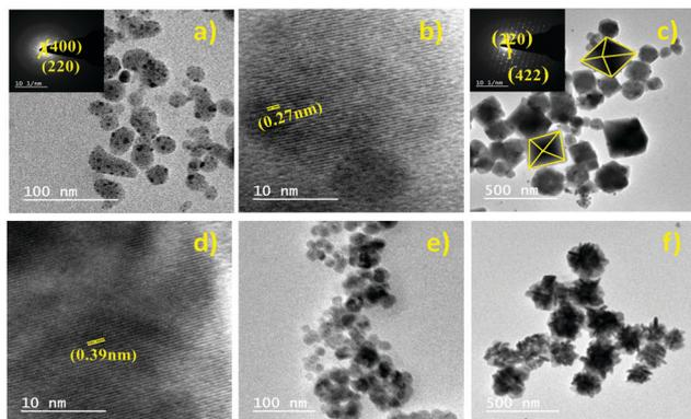
**Fig. 11**  $\text{Cs}_2\text{AgBiCl}_6$  MCs: (a) TEM image (SAED pattern inset) and (b) HRTEM image in organic medium and (c) TEM image (SAED pattern inset) and (d) HRTEM image in aqueous medium.  $\text{Cs}_2\text{AgBiBr}_6$  MCs: TEM images in (e) organic medium and (f) aqueous medium. Reproduced with permission.<sup>76</sup> Copyright 2021, Elsevier.
