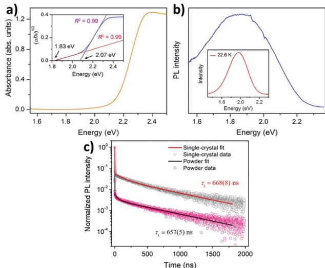
Fig. 7 (a) Absorption spectra, (b) PL spectra and (c) PL decay curves of  $\text{Cs}_2\text{AgBiBr}_6$  double perovskite MCs respectively. Reproduced with permission.<sup>72</sup> Copyright 2016, American Chemical Society.
