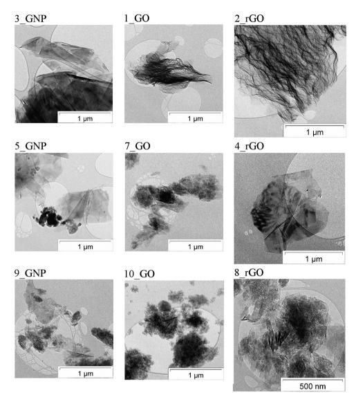
Fig. 2 200 keV TEM images of the 2D carbons. Left column: graphenes, middle column: graphene oxides, right column: reduced graphene oxides.
