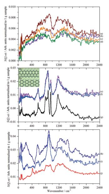
**Fig. 9** TOSCA spectra of the 2D carbon samples after subtraction of the graphite contribution (3\_GNP) grouped by spectral similarity. Top panel: (a) 8\_rGO, (b) 7\_GO, (c) 5\_GNP and (d) 9\_GNP. Middle panel: (e) 2\_rGO, (f) 4\_rGO and (g) glassy carbon<sup>57</sup> (this is not on the same ordinate scale as (e) and (f)). The inset shows H1 and H2 termination. Bottom panel: (h) 12\_GNP, (i) 1\_GO and (j) 10\_GO. Note the different ordinate scales in the panels.
