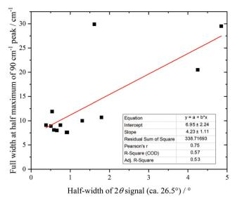
Fig. 11 Correlation of 90 cm $^{-1}$  feature in the INS spectra with the half-width of the XRD peak at 26.5 $^{\circ}$  (002).
