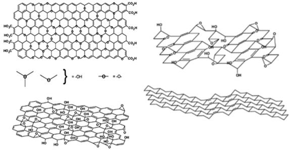
Fig. 13 Structure of graphene oxide as proposed by Lerf and Klinowski<sup>66,67</sup> (left) and Dékány and co-workers<sup>68</sup> (right). In the Lerf-Klinowski model the presence (top) or absence (bottom) of carboxylic acids on the periphery of the basal plane of the graphitic platelets of GO is ambiguous. Reproduced from ref. 3 with permission of the Royal Society of Chemistry.
