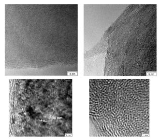
Fig. 3 200 keV TEM images of graphenes showing linear sp<sup>2</sup> type order (i.e. graphite planes - d-spacing 0.34 nm) at the edges (left) and partly turbostratic disorder in the interior (right).
