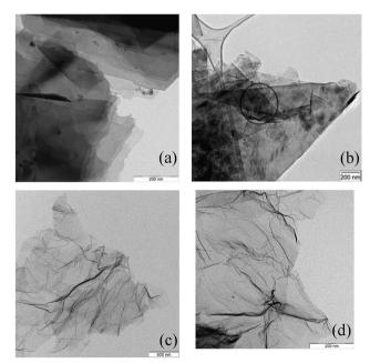
Fig. 4 TEM of GNP ((a) and (b), exfoliated) and rGO (c) and (d), (oxidation and reduction and exfoliation). The dark spots in (a) are inorganic material, the circled area in (b) is partly sp<sup>3</sup>-carbon.
