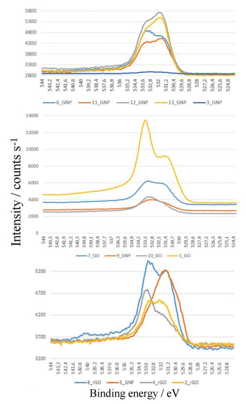
Fig. 6 O1s XPS spectra of the 2D carbon samples.
