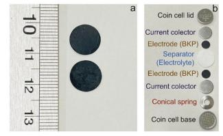
Fig. 2 (a) Self-supporting MWCNT electrodes. (b) Components of a symmetric supercapacitor assembled using a model CR 2032 coin cell filled with the SiWE (7 mol  $kg^{-1}$ ) or WiSE (15 mol  $kg^{-1}$ ) NaClO<sub>4</sub> solutions.
