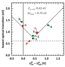
Fig. 11 Lowest optical transition of EDA complexes as function of the intermolecular redox potential difference  $U_{\rm ox}^{\rm D}-U_{\rm red}^{\rm A}$ . The identifiers are taken from Table 1 (green: systems presented here, red: systems from ESI,† and from ref. 9). The solid grey line is fitted following eqn (1).<sup>68</sup> The horizontal line gives the typical lower boundary for optical transitions in EDA complexes from literature at 5000 cm<sup>-1</sup> (0.62 eV). <sup>69,70</sup>
