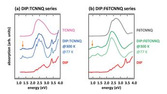
Fig. 4 Absorption spectra for single component and equimolar codeposited D:A films of DIP and TCNNQ (a) as well as of DIP and F6TCNNQ (b). The CT transitions are marked by orange arrows. The absorption spectra for co-deposited D:A were measured at 300 K and at 77 K.
