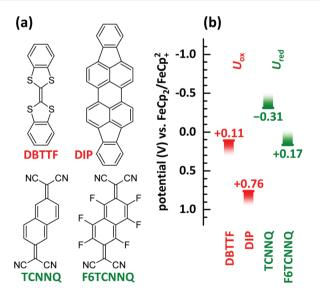
Fig. 3 (a) Chemical structures of donor (DBTTF, DIP) and acceptor (TCNNQ, F6TCNNQ) molecules. (b) Oxidation potentials ( $U_{ox}$ ) of donor and reduction potentials ( $U_{\text{red}}$ ) of acceptor materials determined by cyclic voltammetry. 15,32,33 The oxidation potential for DIP is increased by 350 mV as given in ref. 33 considering the change of the standard potential due to the reported follow up reaction.
