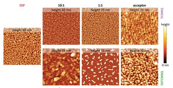
Fig. 7 Scanning force microscopy images (4 × 4 µm²) for single-component and co-deposited D:A films of DIP, TCNNQ and F6TCNNQ. Different height scales are applied and the maximum of the scale is given (upper end of the colour bar at the right side, lower end corresponds to 0 nm). The rootmean square roughness values are 5.8 nm (DIP), 6.2/9.5 nm (10:1), 12.6/11.2 nm (1:1) and 8.2/15.2 nm (TCNNQ/F6TCNNQ), respectively. Image processing was performed using software package Gwyddion.<sup>48</sup>
