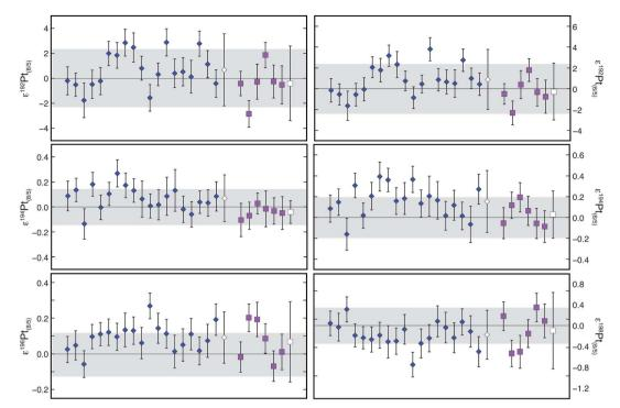
Fig. 2 Mass-independent Pt isotope data for terrestrial reference materials (diamonds = NIST SRM 129c doped with IRMM-010 Pt, squares = Pt- $\alpha$ , open symbols = mean) determined relative to bracketing runs of the IRMM-010 Pt SRM. Error bars denote the  $\pm$ 2se within-run precision; uncertainties of reported means are  $\pm$ 2sd. Grey-shaded area represents the typical between-run precision of the bracketing IRMM-010 Pt runs.
