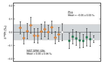
Fig. 6  $\delta^{198}$ Pt values of terrestrial standard reference materials (squares = NIST SRM 129c doped with IRMM-010 Pt, diamonds = Pt- $\alpha$ , open symbols = mean) determined relative to bracketing IRMM-010 Pt SRM runs. Error bars denote the  $\pm 2$ se within-run precision; uncertainties of reported means are  $\pm 2$ sd. Grey-shaded area represents the typical  $\pm 0.06\%$  between-run precision of the bracketing IRMM-010 Pt standard solutions.
