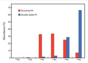
Fig. 1 Isotope composition of the new <sup>198</sup>Pt-<sup>196</sup>Pt double spike. Shown are the double spike Pt isotope abundances, calibrated as described in text (blue bars), in comparison with terrestrial Pt isotope abundances (red bars)
