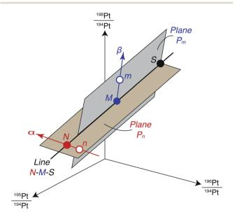
Fig. 7 Schematic of the Pt double spike technique in four-isotope space. Adapted from ref. 35.
