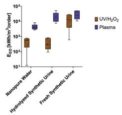
Fig. 4 Calculated electric energy per order ( $E_{EO}$ ) (kW h m $^{-3}$  per order) for both bench-scale reactors in the nanopure water and synthetic urine matrixes. The box and whisker plot displays 95% confidence intervals for  $E_{\rm FO}$  values (n = 6, all pharmaceutical compounds in each data point).
