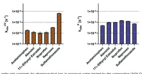
Fig. 1 Observed first order rate constants for pharmaceutical loss in nanopure water treated by the comparative UV/H<sub>2</sub>O<sub>2</sub> system (left) and the experimental plasma system (right).
