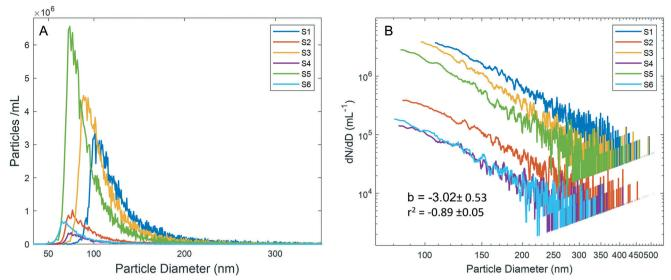
Fig. 2 A) Particle size distributions for <sup>27</sup>Al obtained by spICP-QMS. B) Reprocessed PSD data, with data normalized to number per nm (dN/dD) versus diameter and plotted in log space. The slope (b) and  $r^2$  are an average of all samples; +/-1 SD.
