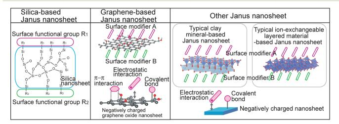
Fig. 1 Structural models of silica-based Janus nanosheets, graphene-based Janus nanosheets and other Janus nanosheets, which exhibited typical nanosheets.
