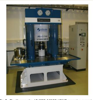
Fig. 2 The Voggenreiter LP 1000-540/50 HP/HT apparatus present in the laboratories of the Institute of Reactor Safety and Nuclear Waste Management (IEK-6), Forschungszentrum Jülich, Germany.
