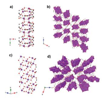
Fig. 12 (a) Crystal structure of  $Gd_2(OH)(suc)_2H_2O\cdot 2H_2O$  with a two-rail Gd-OH ladder parallel to the b-axis and (b) the packing of the ladders on the ac-plane. (c) Crystal structure of  $Gd_6(OH)_8(suc)_5(H_2O)_2\cdot 4H_2O$  showing the three-rail Gd-OH ladder parallel to the b-axis and (d) the packing of the three-rail ladders on the ac-plane. Colour codes: Gd: purple, C: black, O: red. Hydrogens are omitted for clarity.
