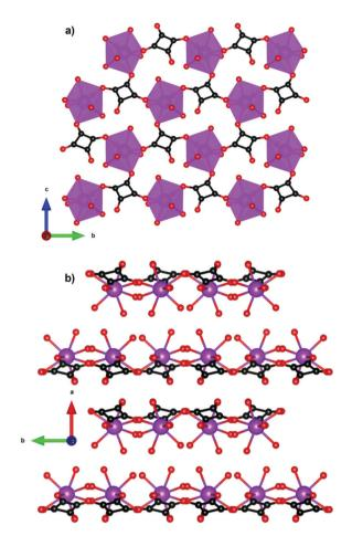
Fig. 14 (a) Two-dimensional layers of Gd(C<sub>4</sub>O<sub>4</sub>)(OH)(H<sub>2</sub>O)<sub>4</sub> on the bcplane and (b) packing of the layers along the a-axis. Colour codes: Gd: purple, C: black, O: red. Hydrogens are omitted for clarity.
