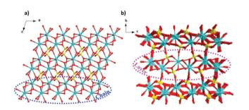
Fig. 4 (a) Crystal structure of Gd(OH)SO<sub>4</sub>, with one-dimensional chains propagating along the a-axis and forming layers along the ac-plane, (b) with the latter stacking along the b-axis. Colour codes: Gd: cyan, O: red, S: yellow. The hydrogen atoms have been omitted for clarity. Reproduced from ref. 60 with permission from the Chinese Chemical Society (CCS), Institute of Chemistry of Chinese Academy of Sciences (IC), and the Royal Society of Chemistry
