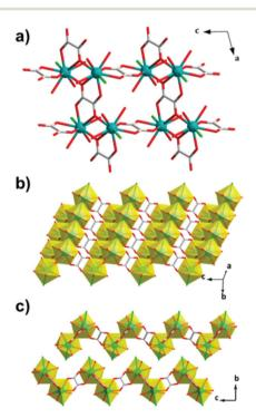
Fig. 10 Crystal structure of Gd(C<sub>2</sub>O<sub>4</sub>)(H<sub>2</sub>O)<sub>3</sub>Cl, with (a and b) 2D layers on the ac-plane and (c) packing along the b-axis. Colour codes: Gd: cyan, C: grey, O: red. The hydrogen atoms have been omitted for clarity. Adapted with permission from Inorg. Chem., 2014, 53(17), 9052-9057. Copyright 2014 American Chemical Society.
