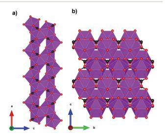
Fig. 5 (a) Crystal structure of  $GdOHCO_3$  with face-sharing  $GdO_{10}$  polyhedra forming zig-zag chains along the a-axis and (b) packing of the distorted triangular lattice along the bc-plane. Colour codes: Gd: purple, C: black, O: red. The hydrogen atoms have been omitted for clarity.
