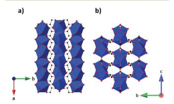
Fig. 11 (a) Crystal structure of Ln(HCO<sub>2</sub>)(C<sub>2</sub>O<sub>4</sub>) with infinite onedimensional chains grow along the a-axis. (b) Arrangement of the chains in a triangular lattice on the bc-plane. Colour codes: Ln: blue, C: black,
