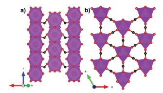
Fig. 9 (a) Crystal structure of Gd(HCO<sub>2</sub>)<sub>3</sub> with chains propagating along the c-axis and (b) arranged in a triangular lattice on the bc-plane. Colour codes: Gd: purple, C: black, O: red. The hydrogen atoms have been omitted for clarity.
