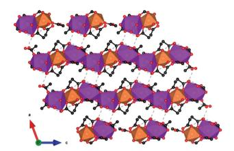
Fig. 16 Crystal structure of  $[GdMn_{0.5}(OAc)_4(H_2O)_2]\cdot 3H_2O$  with chains of Mn and Gd polyhedra bridged together in a 2D network *via* hydrogen bonds. Colour codes: Gd: purple, Mn: orange, C: black, O: red. Hydrogens are omitted for clarity.
