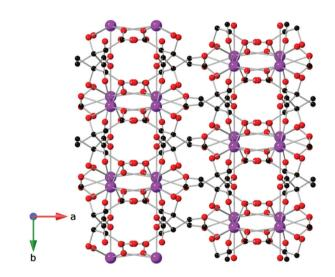
Fig. 13 Two-dimensional layer structure of  $Gd(cit)(H_2O)$  showing two Gd ladder chains propagating along the *b*-axis. Colour codes: Gd: purple, C: black, O: red. Hydrogens are omitted for clarity.
