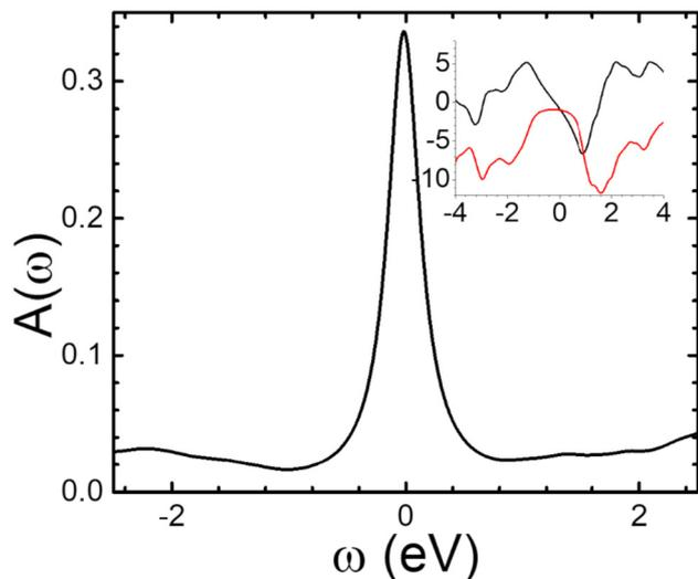
Fig. 4 The spectral function of monolayer MoS<sub>2</sub> at doping 1%. Inset: The corresponding real (black) and imaginary (red) parts of the electron self-energy as function of frequency (both abscissa and ordinate scales have units of eV).
