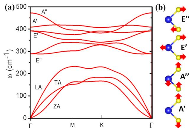
Fig. 3 Phonon dispersion curves (a) and schematic representation of the optical phonon modes (b) for monolayer MoS<sub>2</sub> obtained from DFT calculations.
