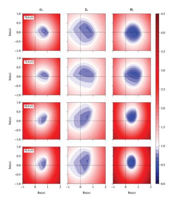
Fig. 5 Contour plots of the spectral radius as a function of the complex parameter  $\omega$  for the **G**,  $\Sigma$  and  $\Pi$  renormalized matrices at 70, 75, 90 and 95 eV.
