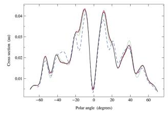
Fig. 6 Comparison of photoelectron diffraction cross sections at 95 eV. Full curve: direct matrix inversion of (I - K); series expansion with **G** renormalization scheme, optimal  $\omega_G$  = 0.790 + 0.124i giving a spectral radius  $\rho(\mathbf{G}_1) = 0.68$ : long dashed curve, truncation order 3; dotted curve, truncation order 5; dash-dotted curve, truncation order 7; dashed curve, truncation order 9
