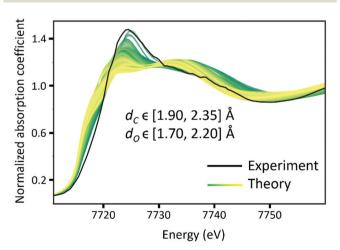
Fig. 8 Comparison between the experimental XANES spectrum of Cocyclam-CO (black) and all the theoretical XANES spectra. The spectra with the colour from green to yellow are simulated XANES with two descriptors changing ( $d_{\mathbb{C}}$  and  $d_{\mathbb{O}}$ )
