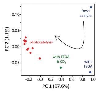
Fig. 4 Plot of 1st and 2nd PCA components of each XANES spectra followed by a K-means clustering (different colours represent different clusters). PC 1 accounts for 97.6% of the total variation around all the spectra, and PC 2 accounts for 1.11%
