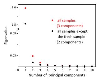
Fig. 3 PCA scree plot showing the result from two sets of XANES spectra, one of all the samples (red) and another one of all the samples except for the fresh sample.
