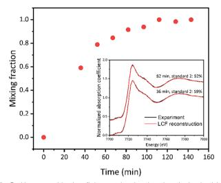
Fig. 5 Linear combination fitting results showing the obtained mixing fraction of standard two. Standard one is the sample with TEOA and CO2 purge before light. Standard two is the sample with light on for 143 min for reaction. Inset shows a comparison between the experimental XANES spectrum and the corresponding reconstruction of XANES spectrum from LCF result at two different reaction times
