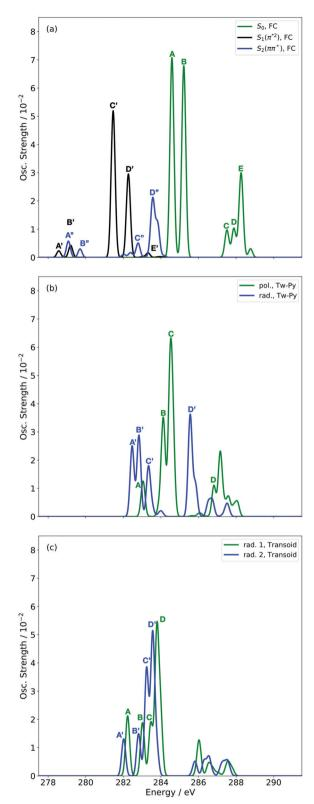
Fig. 4 Simulated XAS at CVS-DFT/MRCI/aug-cc-pVDZ level of theory for  $S_0$ ,  $S_1$  and  $S_2$  states at the FC (a) and key MECI geometries (Tw-Py (b) and transoid (c)) of 1,3-BD.
