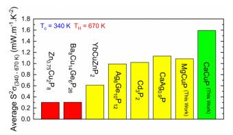
Overview of temperature-average power factor  $\langle S^2/\rho \rangle$  for leading phosphide thermoelectrics. Data taken from: Zn<sub>0.75</sub>Cu<sub>2</sub>P<sub>8</sub>,<sup>11</sup> Ba<sub>8</sub>Cu<sub>14</sub>Ge<sub>6</sub>P<sub>26</sub>,<sup>10</sup> YbCuZnP<sub>2</sub>,<sup>8</sup> Ag<sub>6</sub>Ge<sub>10</sub>P<sub>12</sub>,<sup>6</sup> Cd<sub>3</sub>P<sub>2</sub>,<sup>13</sup> CaAg<sub>0.9</sub>P. <sup>14</sup>
