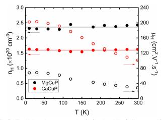
Fig. 3 The Hall carrier concentration ( $n_{\rm H}$ ) and mobility ( $\mu_{\rm H}$ ) between 10-298 K, demonstrating that the hole concentration is independent of
