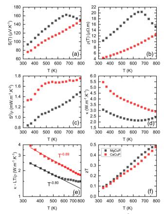
Fig. 2 Temperature dependence of (a) S(T), (b)  $\rho(T)$ , (c)  $S^2/\rho(T)$ , (d)  $\kappa(T)$ , (e)  $\kappa_{\rm lat}(T)$  and (f) the figure of merit, zT for MgCuP (black) and CaCuP (red) between 300–800 K.
