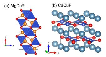
Fig. 1 Crystal structures of (a) MgCuP and (b) CaCuP. Mg = orange, Ca = turquoise, Cu = blue and P = red. In MgCuP, edge linked CuP<sub>4</sub> tetrahedra form chains aligned in the b direction
