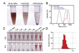
Fig. 2 Characterization of B-Au NPs after Boc deprotection by different methods. (A) Photos of B-Au NPs and the resulting deprotected Au NPs. (B) DLS analysis of B-Au NPs and the resulting deprotected Au NPs. (C) Images of T-Au NPs, B-Au NPs, and TB-Au NPs with different T/B ratios synthesized with a ligand exchange reaction. (D) Average diameter of Au NPs tested by DLS.
