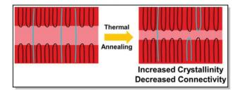
Fig. 4 The effect of postdeposition thermal annealing on P3HT\_40 Reproduced with permission from American Chemical Society.<sup>74</sup>
