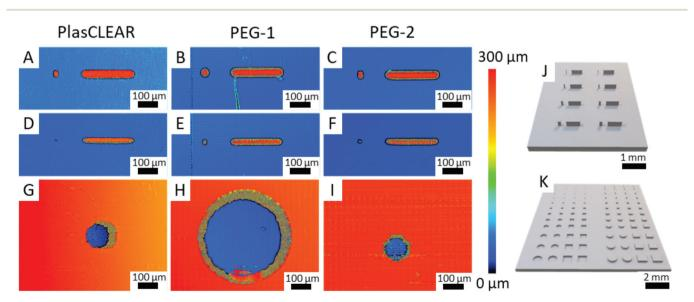
Fig. 7 CLSM height images of printed pillars, walls (A–F) and holes (G–I). With all three resin, a minimum pillar size of 50  $\mu$ m (A–C), and minimum wall size of 35  $\mu$ m (D and E) could be printed. Minimum hole size varies with resin, and is 120  $\mu$ m for PlasCLEAR (G), 370  $\mu$ m for PEG-1 (H) and 100  $\mu$ m for PEG-2 (I). CAD models for testing the maximum resolution for freestanding pillars and walls (J) and holes (K).
