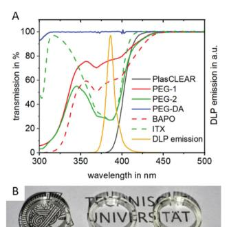
Fig. 2 UV/VIS photospectroscopy of all resins and their single components shows the transmission of light at wavelengths between 300 and 500 nm (left y-axis), with the printer's DLP emission spectrum (right v-axis) showing a clear peak at 385 nm (A). Images of printed cell culture dishes of all printing materials show the high post-printing transparency for all three selected resins (B).
