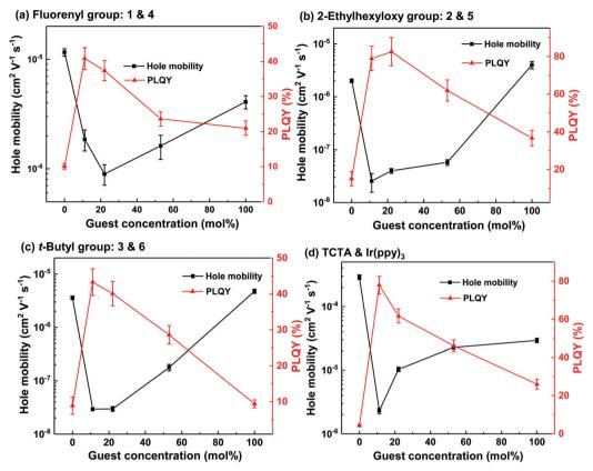
Fig. 4 Mobility and PLQY values of neat and blend films of **1** and **4** (a), **2** and **5** (b), **3** and **6** (c) and TCTA and Ir(ppy)<sub>3</sub> (d) at different concentrations. Fig. (d) was reproduced with permission.<sup>26,27</sup>
