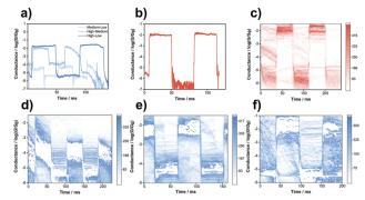
Fig. 2 (a and b) Sample traces of **TPE-m-OH** and **TPE-p** for conductance changing with the compression–elongation of piezo. (c) A 2D histogram constructed from selected traces for **TPE-p**. (d–f) A 2D histogram was constructed from selected traces for **TPE-m-OH** for conductance switching between (d) medium and low conductance, (e) high and medium conductance, and (f) high and low conductance.
