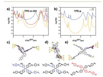
Fig. 4 (a and b) Calculated transmission spectra for TPE-m-OH (a) and **TPE-p** (b) with different anchoring sites. (c-e) The transmission path for  $S_1-S_4$  (c), the  $N_1-N_4$  anchoring site of **TPE-m-OH** (d), and the  $S_1-S_4$ anchoring site of TPE-p (e).
